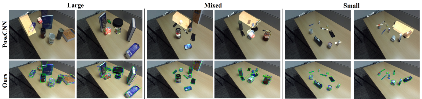
Fig. 3: Comparing predictions from PoseCNN [5] (top row) and our approach (bottom row) on a set of tabletop images, splitting objects into three bins according to their size (3D bounding box volume). Ground truth bounding boxes are green, predictions blue.
