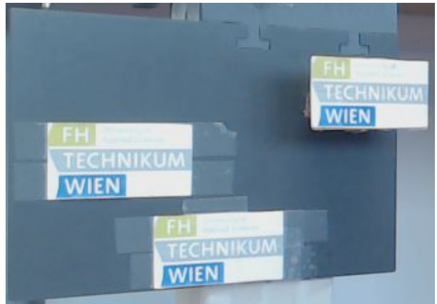
Figure 1. The visual target used for docking. The target location is on the ground in front. The origin for the PnP solvers is in the upper left corner. The logos are roughly 9x3 centimeters in size. The upper right logo was raised during experiments to remove coplanarity.
