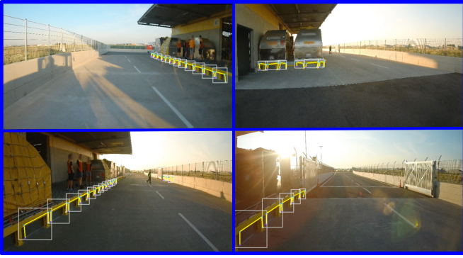
Fig. 5. Example results for detecting ramp structural elements (as defined in Fig. 3) via a set of key-points. Note the varying illumination and viewing conditions.
