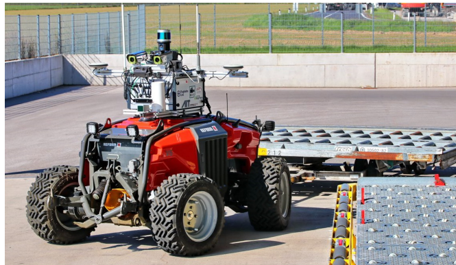
Fig. 4. The employed mobile platform (Reform-Werke Metron P48 RC) equipped with multi-sensor and control hardware.
